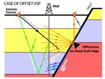
A Vertical Seismic Profiling is a field measurement procedure in which the seismic source is activated at a fix surface position and the seismic signal recorded by sensors located in a well at successive depth levels.
