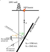
P-S reflections from highly dipping fractured corridors, confirmed by the well logs.
